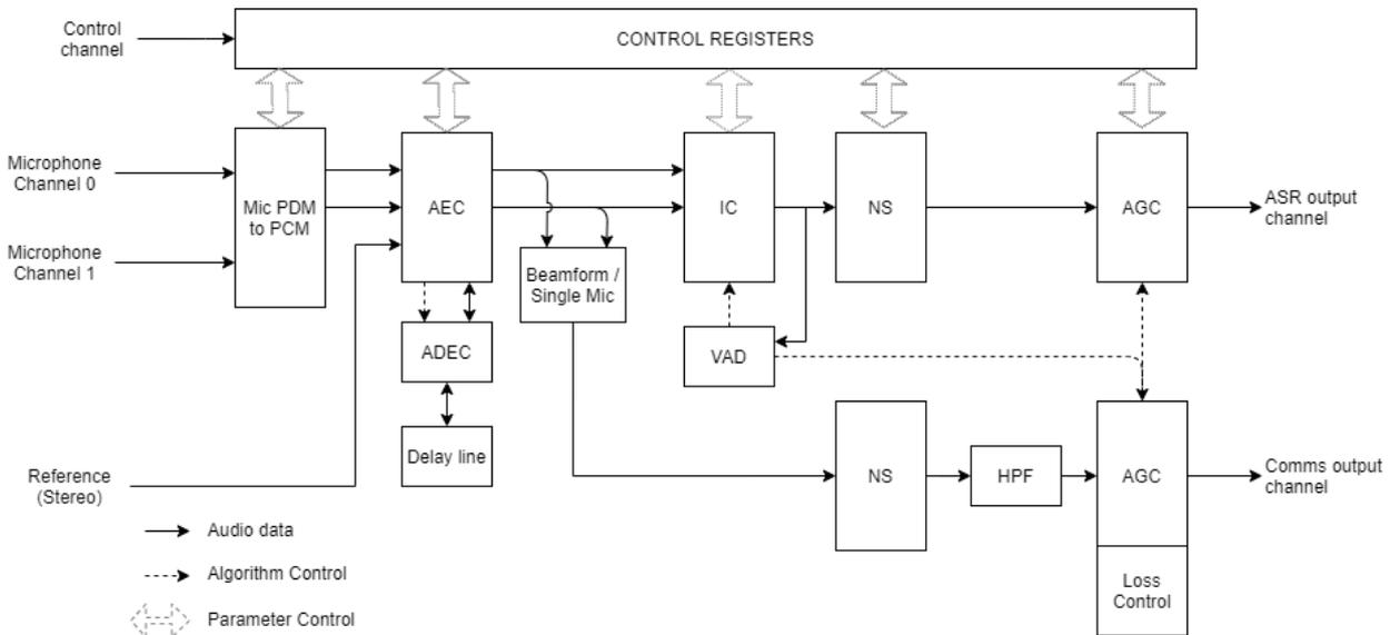
Fig. 3.1: The XVF3615 audio processing pipeline
