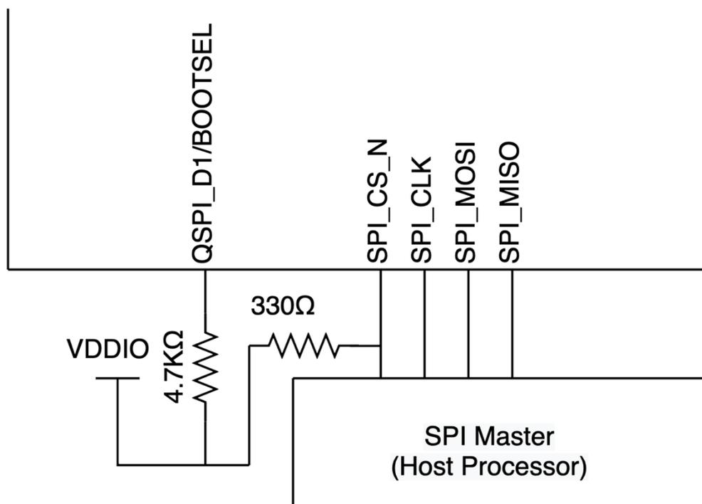
Fig. 5.2: XVF3615 SPI Slave boot configuration
