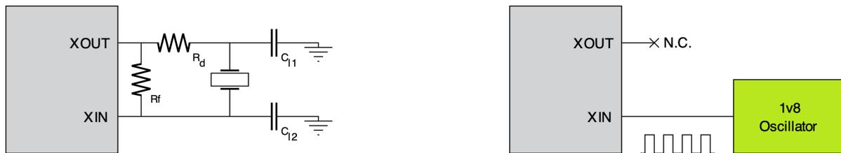
Fig. 6.1: Crystal oscillator or clock input configurations
