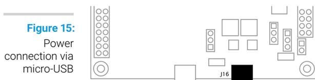
The voltage is converted by the on-board regulator to the 1V and 3V3 supplies used by the components. Additional or alternative power sources may use the power headers provided as shown in Figure 16:
