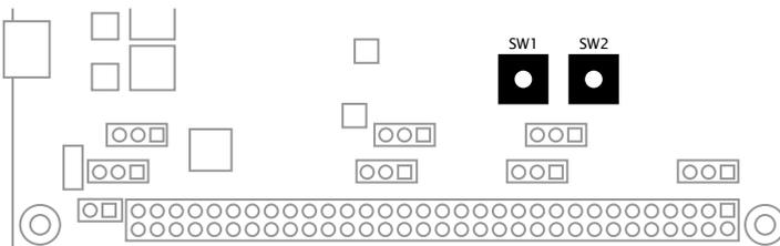
Each push-button switch is connected to a different IO on the xCORE-200 device as described in Figure 9:
