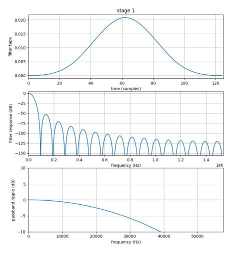
Fig. 3: First stage decimation filter freq response
