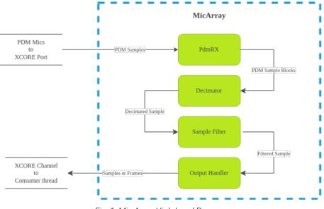
Fig. 1: Mic Array High Level Process
