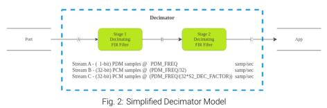
The first stage filter is a decimating FIR filter with a fixed tap count (S1\_TAP\_COUNT) of 256 and a fixed decimation factor (S1\_DEC\_FACTOR) of 32.
