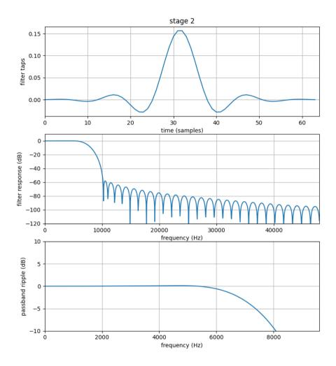
Fig. 4: Second stage decimation filter freq response
